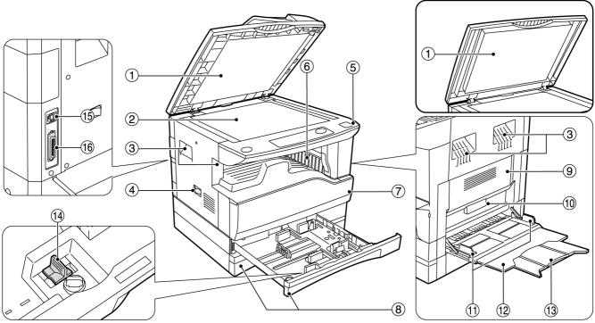
① Document feeder cover (when the ADF is installed) /document cover
